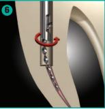
6. Twist assembly in a "to and fro" motion until the obstruction starts to give. Continue to rotate and lift in a counter-clockwise motion to remove obstruction.
